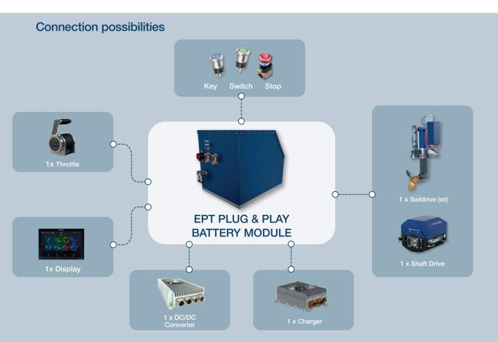
Input possibilities: 1 propulsion unit (1 x saildrive or 1 x shaftdrive)Battery system: 18.2 kWh or 36.7 kWh battery units with 100 VDC
