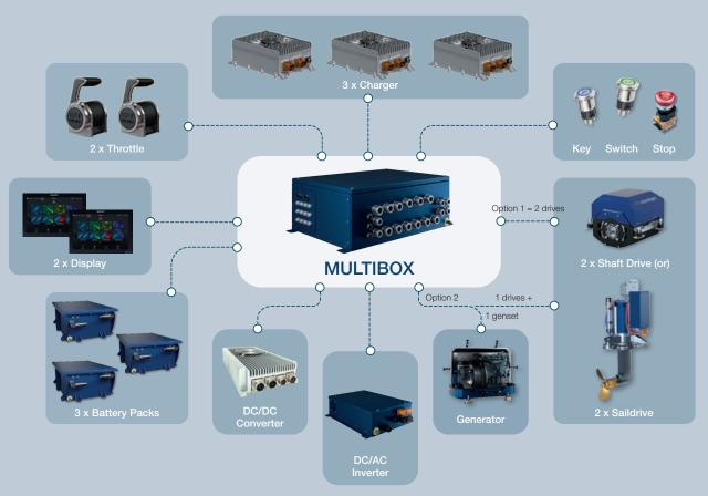
**Input options:** 2 propulsion units (2 x sail drive or 2 x shaft drive) OR:
